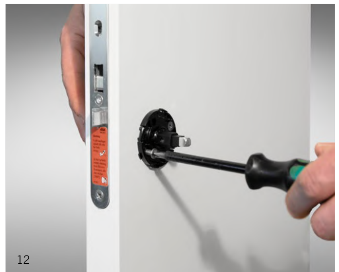
Image 12 Insert and tighten the screws supplied from the righthand side of the door. On the left- hand side, use the other hand as a means of holding the bearing in position. The sleeves are fitted from the lefthand side.
