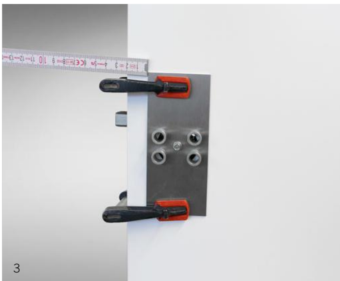
Image 3 Lining the drilling template up: parallel with the edge of the door.
